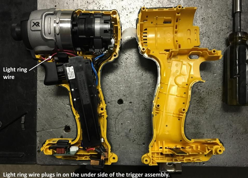
Light ring wire plugs in on the under side of the trigger assembly.
