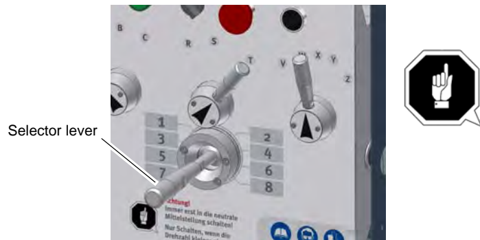
Fig. 4-5: Feed selection lever
