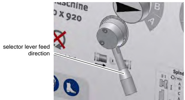
Illustr. 4-7: selector lever feed direction
