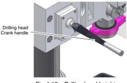
Fig.4-12: Drilling head height adjustment
