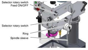
Fig.4-8: Selector rotary switch sleeve feed
