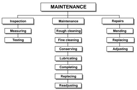
Fig.7-1: Maintenance - Definition according to DIN 31051
