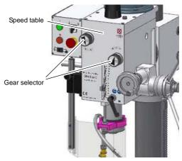
Fig.4-5: Gear selector
