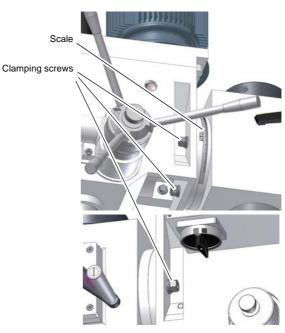
Fig.4-10: Clamping screws drilling head
