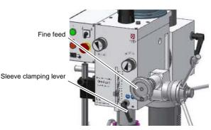
Fig.4-9: Sleeve clamping lever
