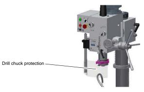
Fig. 1-5: Drill chuck protection
