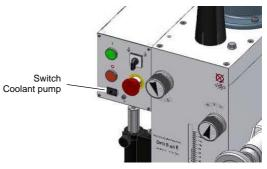
Fig.4-21: Switch cooling unit
