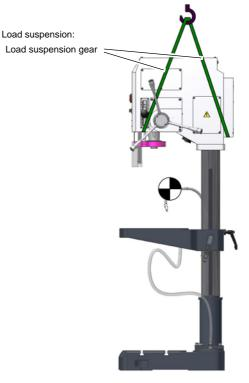
Fig.3-1: Example of load suspension and of lifting loads
