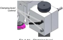
Fig.4-11: Clamping lever/ Locknut drilling head
