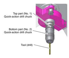
Fig. 4-15: Quick-action drill chuck
