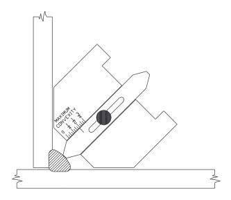
After the size of a convex weld has been determined, place the gauge against the structure and slide pointer until it touches face of the fillet weld has shown.
