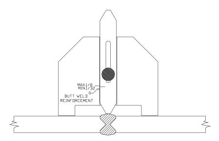
Place gauge so that reinforcement will come between legs of gauge and slide pointer out until it touches the face of weld has shown.
