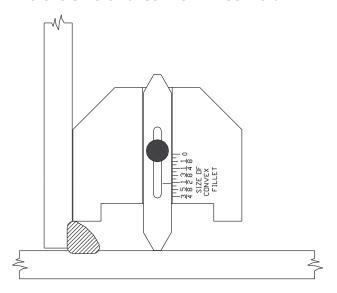
Place gauge against the toe of the shortest leg of the fillet and slide pointer out until it touches structure as shown. Read "size of convex fillet" on face of gauge.
