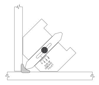
Place gauge against structure and slide pointer out until it touches the face of the fillet weld as shown. Read "size of concave fillet" on face of gauge.
