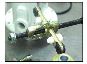
B. Grease heavily and place the trip rod (40) into the air motor piston (34) with the stems of the poppet valves (32\*) going through the lower valve grommets (17\*).
