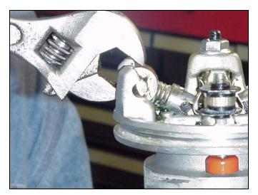
30. Swing the toggle assembly up and away from the piston lugs, and remove the assembly.
