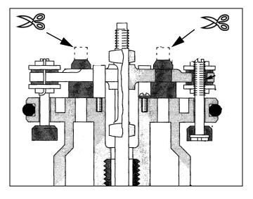
5. Place the poppet valves (32\*) in the air motor piston (34).
