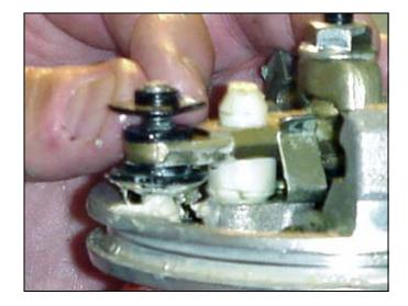
11. Install the toggle pins (36) in the trip rod yoke (23).
