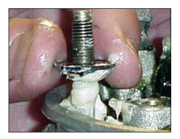
7. Assemble the trip rod yoke (23) and actuator valve (27) and insert the trip rod (40).
