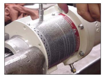
20. Remove the six hex head cap screws (9) holding the air motor cylinder (35) to the air motor base (28).
