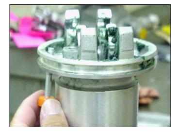
Thread the bottom valve nuts (24\*) onto the stems of the poppet valves until there are a few threads left before the threads run out.
