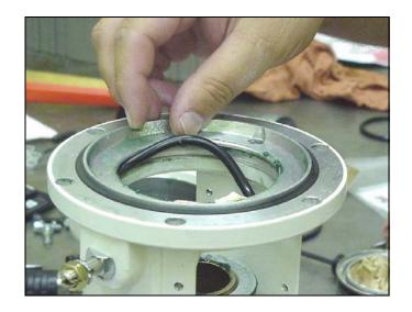
19. Grease and install the new o-ring packing (12\*).
