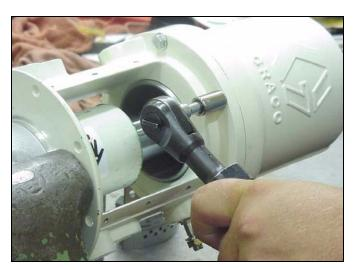
Carefully pull the air motor cylinder (35) straight off of the air motor piston (34).
