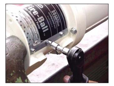
30. Replace the six screws (7) holding the warning plate (47) onto the air motor base (28).
