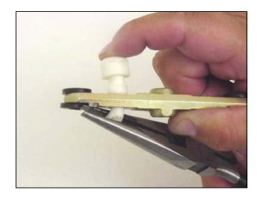
Clip off the top parts of the valve poppets (31\*) shown with dotted lines.
