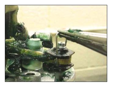
34. Screw the top valve nuts off (24\*).
