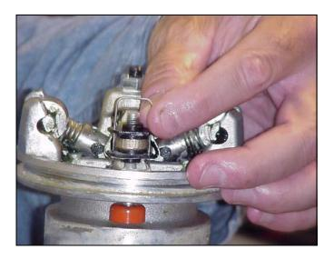
Pull the lock wires (25\*) down tightly, and bend the ends out with pliers so that they cannot be pulled back out of the holes.
