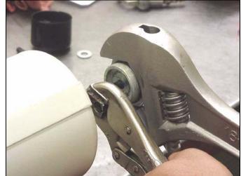
17. Thread the service nut (A) (not supplied) onto the top of the trip rod (40).
