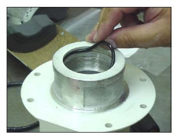
24. Remove the block packing (16\*) from the bottom of the air motor base (28).
