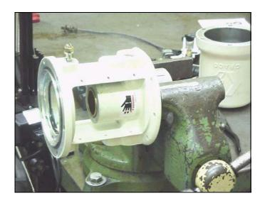
22. Grease the outside of the air motor piston (34) and displacement rod (29).
