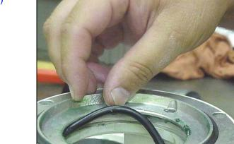
25. Remove the o-ring packing (13\*) from the air motor base.
