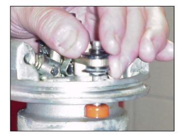
Align the holes in the valve nuts (24\*) and the slots on the stems of the poppet valves (32\*) and install the lock wires (25\*) through the holes in the top and bottom valve nuts. For more detail see FIG. 1, page 36.
