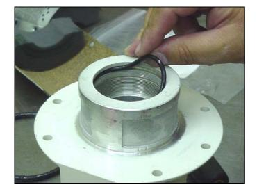
Install the new block packing (16\*) through the bottom of the air motor base (28), with the lips facing toward the bottom of the pump.
