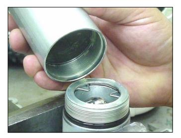
Remove ball retainer and inspect the metallic ball (8), ball retainer (44), and seat of valve housing (42) for damage.
