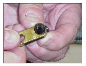
3. Pull the new poppet valves (31\*) into the valve actuator (27).
