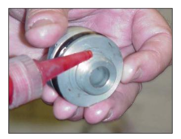
34. Thread the fluid piston (43) onto the displacement rod (29). Torque to 40 to 60 ft-lb (54 to 81 N.m).
