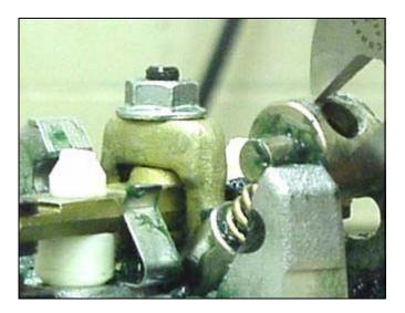
13. Set gap using the gap adjustment tool\*.
