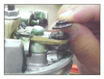
35. Pull the valve assembly out of the piston.
