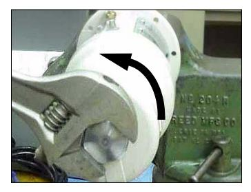
14. Pull up on the cylinder cap nut (39) to expose the trip rod (40).
