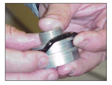
Clean the threads of the fluid piston (43) and apply Loctite to the threads.
