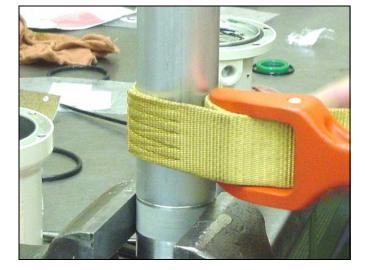
2. Horizontally clamp the air motor base (28) in a vise by closing the vise jaws on the air motor flange.
