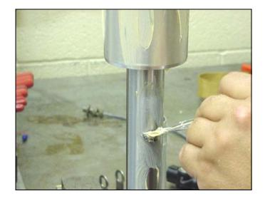
23. Slide the displacement rod (29) through the packings, and slide the air motor piston (34) into the air motor base (28).
