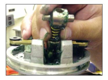
Remove the toggle pins (36) from the trip rod yoke (23).
