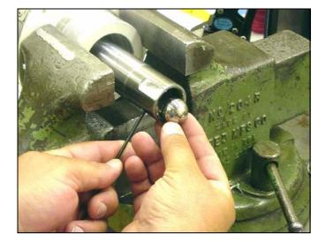
32. Install the new o-ring packing (11\*) onto the fluid piston.
