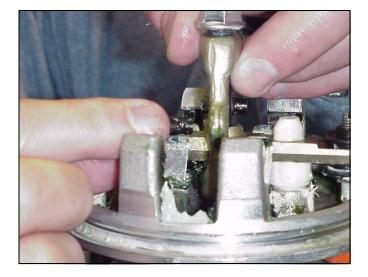
12. Place the toggle arm (38) ends of the toggle assembly onto the toggle pins (36), and snap the pivot pin ends of the toggle assembly into the piston lugs.
