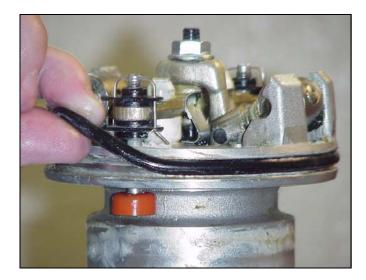
18. Grease and install the new o-ring packing (13\*).
