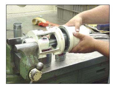
Replace the six button head screws (9) holding the air motor cylinder (35) to the air motor base (28).
