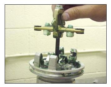
36. Remove the trip rod (40), trip rod yoke (23), and valve actuator (27).
