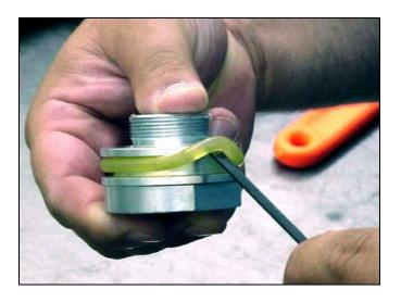
13. Unscrew the cylinder cap nut (39) from the top of the air motor cylinder (35).
