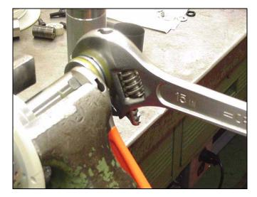
Remove the metallic ball (6) from the end of the displacement rod (29).
