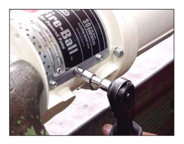
19. Remove the six hex head screws(7) holding the warning plate (47) to the air motor base (28).
