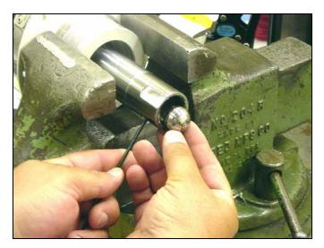
12. Remove the packing o-ring (11\*) from the fluid piston (43).
