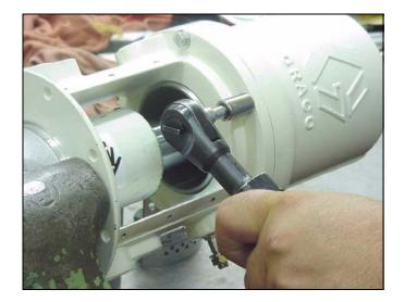
Remove the nut (A) on the trip rod (40) and grip the trip rod with padded pliers (see page 5).
