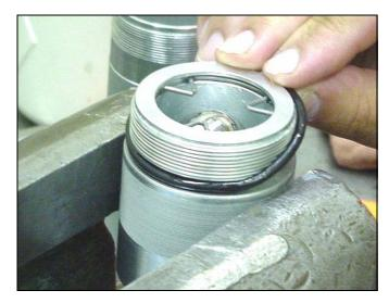
7. Remove and replace the o-ring packing (21\*).
