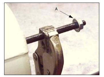
27. Tighten the cylinder cap nut (39).
