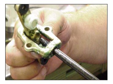
37. To remove the valve poppets (31\*) cut them with a sharp knife or side cutter.
