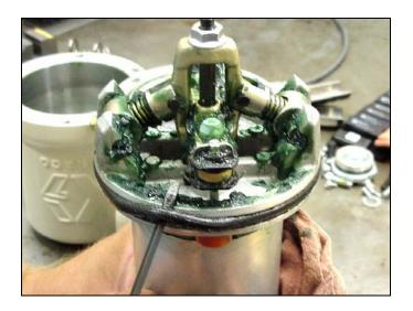
Use a screwdriver handle to push down the trip rod yoke (23) to snap the toggle arms (38) down.
