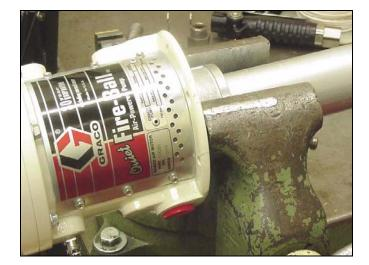
Use a strap wrench or chain wrench on the fluid cylinder (41) to screw it out of the air motor base (28).
