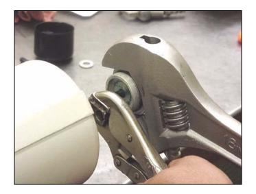
28. Screw the cylinder cap (39) onto the top of the cylinder.
