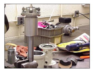
27. Remove the o-ring packing (18\*) from the air motor piston (34).
