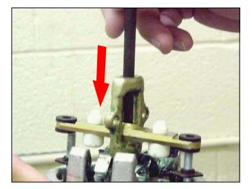
Check that the valve actuator (27) is aligned by the spring clips (26), and slides easily into them. Replace the spring clips (26) if worn or bent.
