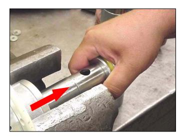
10. Using wrenches on the flats of the displacement rod (29) and on the flats of the fluid piston (43), unscrew the fluid piston from the displacement rod.
