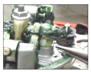
Remove the lockwires (25\*) from the valve nuts (24\*).
