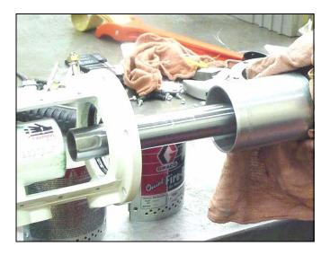
24. Carefully slide the air motor cylinder (35) straight onto the air motor piston (24).
