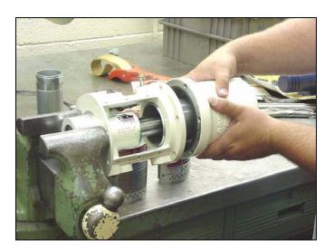
22. Pull the air motor piston/displacement rod assembly (34, 29) clear of the air motor base (28).
