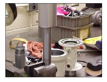
Install the new lower valve gromments (17\*) in the valve actuator (27).
